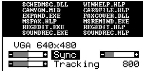
A quiet, interference-free image is projected in a range of several settings. Set the LCD monitor to approx. the middle of this range. The following image appears when the **Sync** setting is correct:
