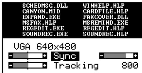
An automatic synchronisation adjustment can be called up with the **Select** key. Afterwards the Sync found setting is displayed on the screen.
